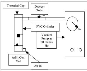
The Draeger-Tube<sup>TM1</sup> detects arsine gas in air. The distance that a purple color travels up the tube quantifies the amount of arsine present. Samples containing 500  $\mu$ g/L arsenic were tested using both methods. The Hach method uses a 50 mL sample and the competitor uses a 5 mL sample. The vacuum pump was set at 20 inches of Hg and allowed to run continually for the full 30 minutes of each test. The results of the experiment are shown here.
